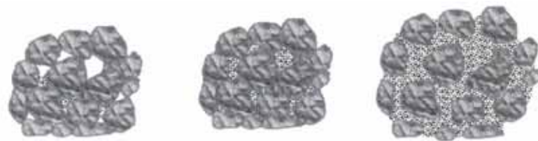
a) Low SS (Unstable) b) Optimum SS (Stable) c) Excess SS (Disrupted)
