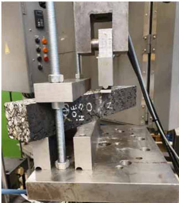
Cantilever shear test
