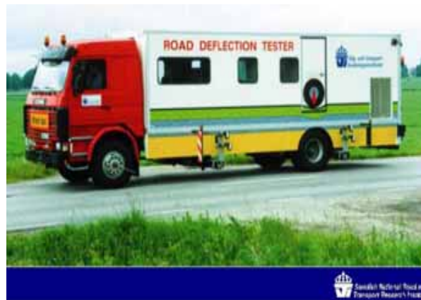
Rolling Wheel Deflectometer (RWD)
